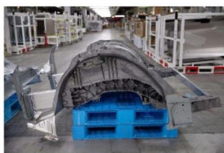
Model Y rear underbody 2 pieces of metal (eventually a single piece)
