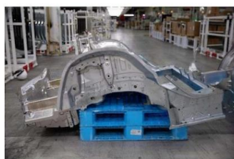
Model 3 rear underbody 70 pieces of metal
